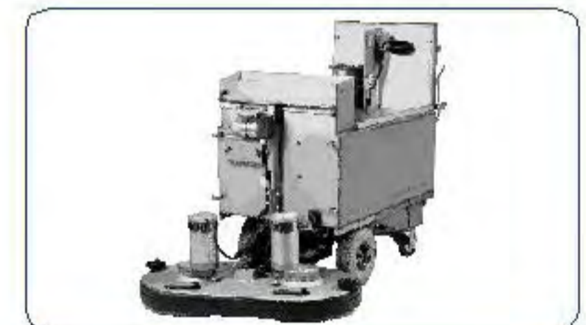
Sturdy and reliable self-supporting AISI 304 stainless steel tank.
